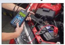
Using the optional Amp Clamp provides an enhanced level of diagnostics beyond just starter voltage drop. The EXP starter diagnostics include starter amps draw, voltage drop, start time, and starter circuit resistance resulting in more accurate results.
