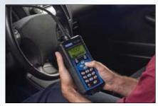
From battery, starter, and alternator diagnostics to circuit integrity testing, the EXP is the most versatile and reliable electrical diagnostic tool on the market today. With the ability to perform more tests with one tool, you can be more efficient, cut costs, and easily update to the newest technologies
