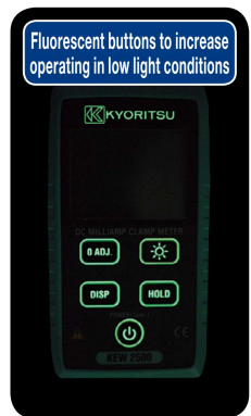
Diameter of measurable conductor : φ6mm max
