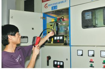
This high-definition video borescope has 2.4 "TFT LCD, Resolution: 480 (W) X234 (H), applying H.264 video codec technology makes images clear and exquisite, and equipped with curved waterproof goose-shaped tube which is a meter long, it will be easy to detect the object that cannot be touched and can't be visible by naked eye, meanwhile, access to AV video display and the signal system can be derived in both NTSC / PAL formats and can switch the signal format automatically.
