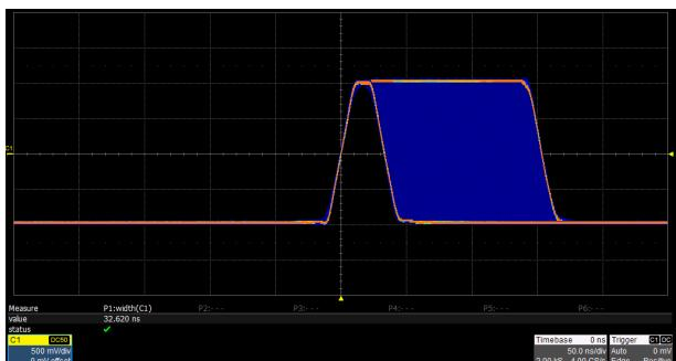
The rise/fall times can be set independently to the minimum of 16.8 ns at any frequency and to the maximum of 22.4 s. The adjustment step is as small as 100 ps. The Pulse width can be fine-tuned to the minimum of 32.6 ns with the adjustment step as small as 100ps.
