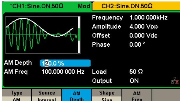
Multiple modulation types: AM, DSB-AM, FM, PM, FSK, ASK, PSK and PWM. The modulation source can be configured as "Internal" or "External".
