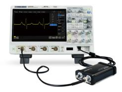
the SDS5000X can control the SAG1021 USB Function/Arbitrary waveform generator to output waveform with up to 25 MHz frequency and  $\pm 3$  V amplitude. Six basic waveforms plus multiple types of arbitrary waveforms are built-in
