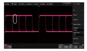
With a waveform update rate of up to 110,000 wfm/s, the oscilloscope can easily capture unusual or low-probability events. In Sequence mode the waveform capture rate can reach 480,000 wfm/s
