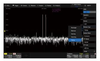
Hardware accelerated FFT supports up to 2 Mpts operation. This provides high frequency resolution with a fast refresh rate. The FFT function also supports a variety of window functions so that it can adapt to different spectrum measurement needs. Three modes (Normal, Average and Max hold) can satisfy different requirements for observing the power spectrum
