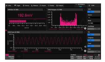
4-digit voltmeter and 7-digit frequency counter. Any analog channel can be selected as a source. Bar, Histogram and Trend diagrams are supported
