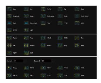
Parameter measurements includes 3 categories: horizontal, vertical and CH delay providing a total of 39 different types of measurements. Measurements can be performed within a specified gate period. Measurements on Math, Reference and History frames are supported
