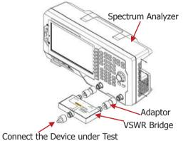
Connect the device under test
