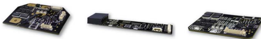
BMS test board
