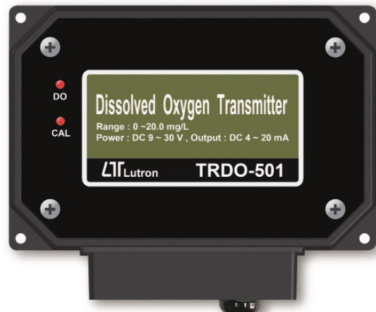
4 to 20 mA, IOT transmitter DISSOLVED OXYGEN TRANSMITTER Model : TRDO-501 * Please contact LUTRON for detailed catalog.
